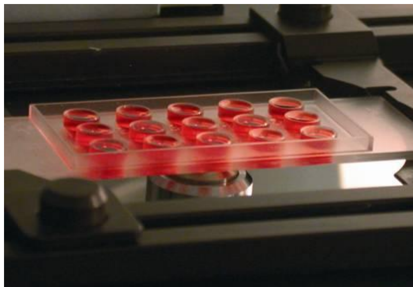
Assay tray to optically select and measure successful microbe cultures
